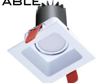
The Alta Adjustable LED is a 130 x 130mm square downlight which uses a CREE LED engine. The heatsink is constructed from die-cast aluminium complete with and adjustable aluminium bezel and reflector. The bezel features a 40mm recess detail creating a glare friendly cut-off which is also an aesthetically pleasing architectural detail.
