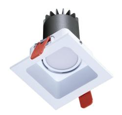
The Alta Mini Adjustable LED is a 90 x 90mm square downlight which uses a CREE LED engine. The heatsink is constructed from die-cast aluminium complete with an adjustable aluminium bezel and reflector. The bezel features a 40mm recess detail creating a glare friendly cutoff which is also an aesthetically pleasing architectural detail.
