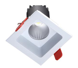
The Alta LED is a 130 x 130mm square downlight which uses a CREE LED engine. The heatsink is constructed from die-cast aluminium complete with aluminium bezel and reflector. The bezel features a 40mm recess detail creating a glare friendly cut-off which is also an aesthetically pleasing architectural detail.
