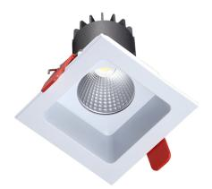
The Alta Mini LED is a 90 x 90mm square downlight which uses a CREE LED engine. The heatsink is constructed from die-cast aluminium complete with aluminium bezel and reflector. The bezel features a 40mm recess detail creating a glare friendly cutoff which is also an aesthetically pleasing architectural detail.
