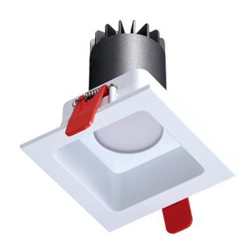
The Alta IP LED is a 130 x 130mm square downlight which uses a CREE LED engine. The heatsink is constructed from die-cast aluminium complete with aluminium bezel and reflector. The bezel features a 40mm recess detail creating a glare friendly cut-off which is also an aesthetically pleasing architectural detail.
