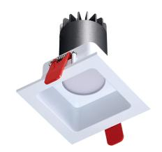
The Alta Mini IP LED is a 90 x 90mm square downlight which uses a CREE LED engine. The heatsink is constructed from die-cast aluminium complete with aluminium bezel and reflector. The bezel features a 40mm recess detail creating a glare friendly cutoff which is also an aesthetically pleasing architectural detail.
